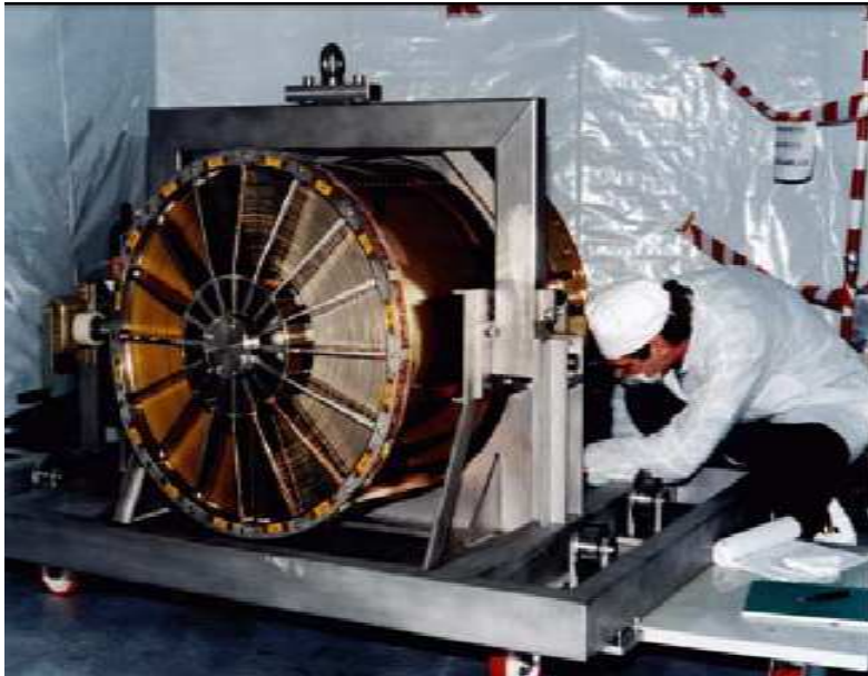
One of the three modules of the XMM-Newton Mirror Assembly
