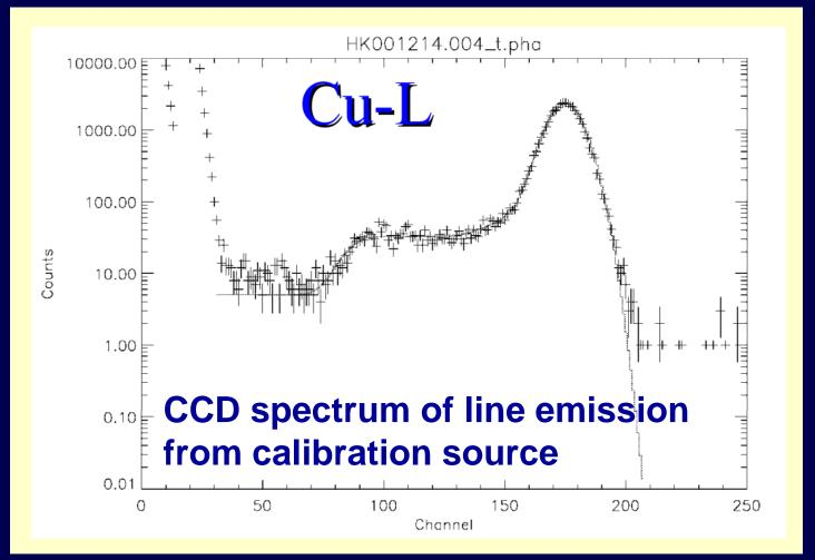
Monochromatic X-ray photons can induce different signal charges
