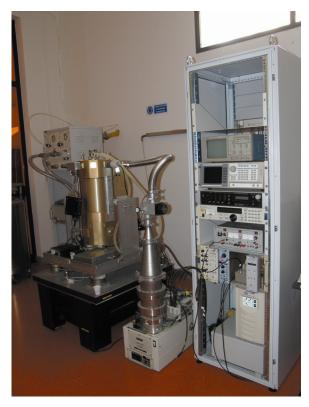
Fig. 2. The cryostat used for developing low temperature detectors.
