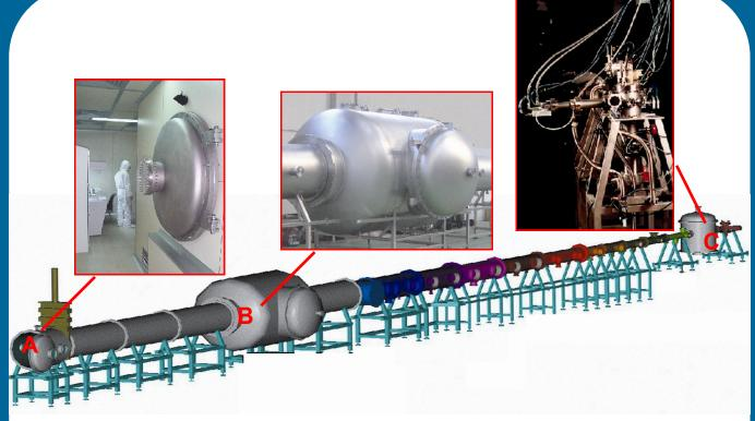
**Fig. 1.** Diagram showing the high-vacuum tube at the XACT laboratory: **A** The high vacuum chamber door, accessible from the clean room. **B** The chamber for X-ray telescope testing. **C** The X-ray source.
